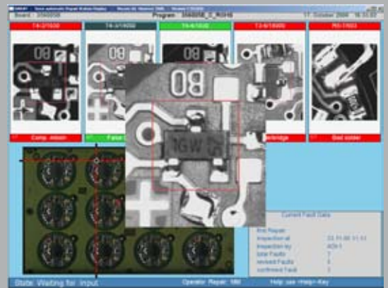
Overview photograph and close-up of single inspection defects
