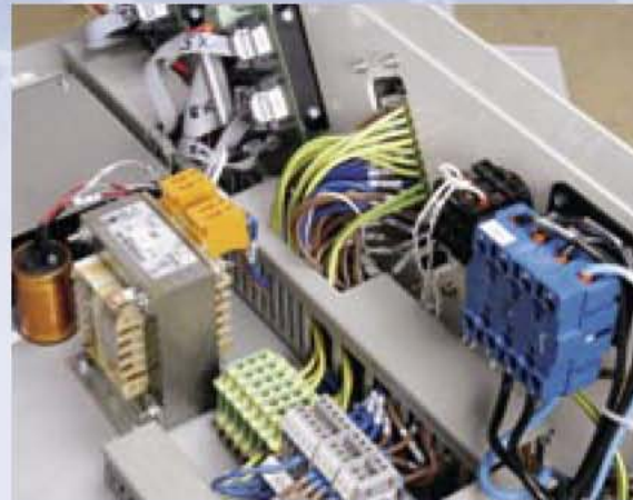
Compact a modern control system with interfaces for binary coding, barcode and transponder.
