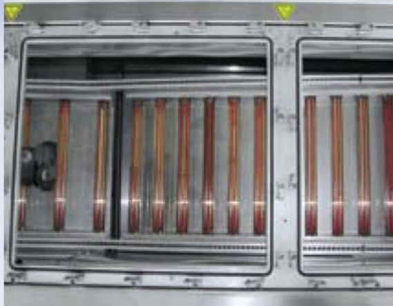
Infrared and carbon emitters allow an optimal preheating, independent of alcohol- or water based flux.
