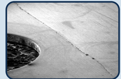
Photo shows crack in a nickel blade undetectable to the eye.
